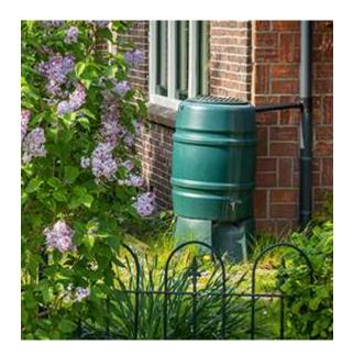
A basic rain barrel **collects water from a downspout** (ensure you have a diverter for when the barrel gets full) **with a water outlet on the lower portion** of the barrel. **Elevating the barrel** helps the water flow. Some rain barrels also have an option to connect multiple barrels to collect more rainwater.
